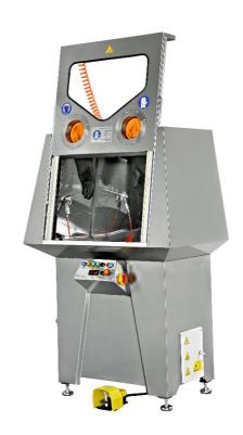
The Washkleen MC160, MC180 and MC200 give a choice of fully enclosed manual parts wash stations all constructed from stainless steel. Their wash chambers are accessed from the front for ease of loading and foot print savings. The machines are fitted with high-pressure spray guns that are controlled from a foot pedal allowing the operator to keep both hands free making these machines ideally suited for cleaning more heavily soiled components.
