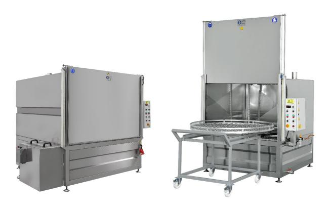
The **WashKleen F1250** and **F1500** are a good choice for medium to heavy duty component cleaning and degreasing applications. These front-loading spraywash machines are of stainless steel construction, the heated wash solution is sprayed onto the components from the top, bottom and side delivered from the rotating spray boom achieving an extensive wash coverage. The loading trolley with its roll in-out basket makes easy work of handling heavier loads.
